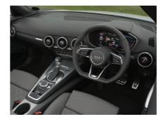
LCD display that fills the instrument binnacle and replaces the traditional analogue dials. You can choose between two display modes: in the classic view, the speedometer and rev counter are in the foreground; in 'infotainment' style the virtual instruments are smaller. The space that becomes free as a result provides plentiful room for other functions, such as the very clear navigation map.
